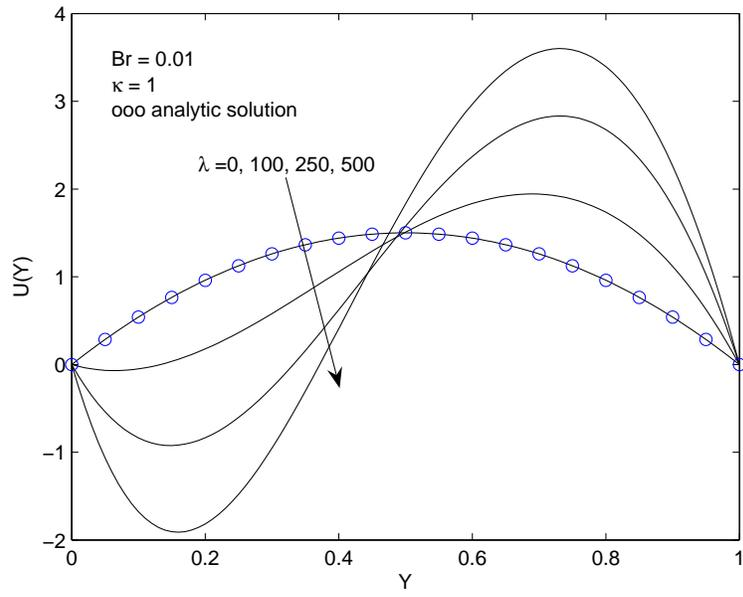
Figure 2: Velocity profiles for different values of  $\lambda$
