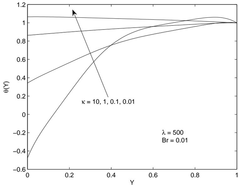
Figure 7: Temperature profiles for different values of  $\kappa$
