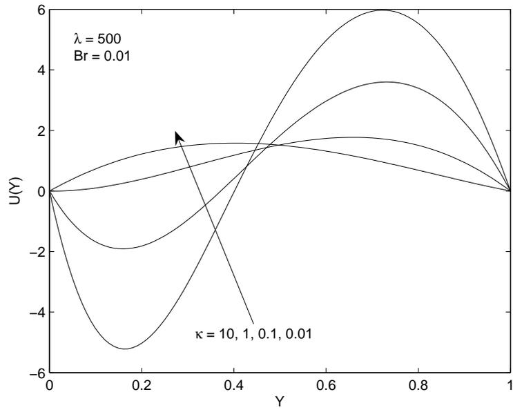
Figure 4: Velocity profiles for different values of  $\kappa$
