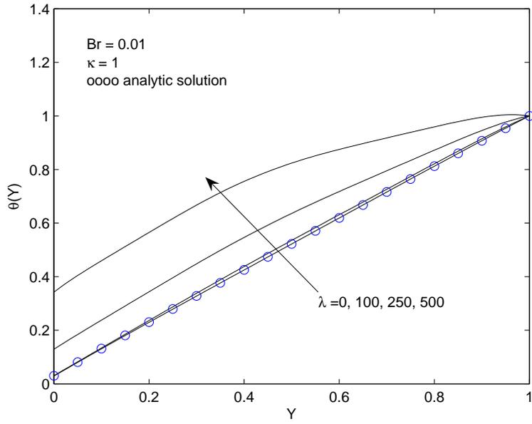
Figure 5: Temperature profiles for different values of  $\lambda$
