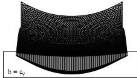
Fig. 6. Deformed mesh and contact interface forces for b = c_v
