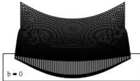
Fig. 7. Deformed mesh and contact interface forces for b = 0
